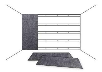
3. Same as installation 2, but mineral wool (same thickness as battens) is placed between the battens.
